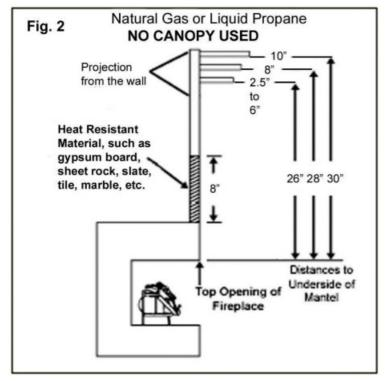
**NOTE:** A hood (canopy) as shown in Fig 3 is used to deflect heat away from the fireplace face and mantle, reducing the chances of heat damage or discoloration. If using a hood, it must project a minimum of 4" from the
