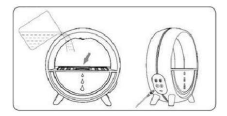
Power Button: Press and hold for 3 seconds to tum on or off the humidifier and the ambient light, and the humidifier starts to pump water and spray.
