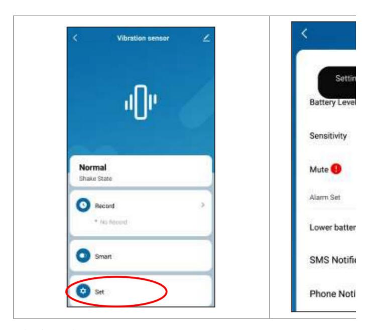
2). Set->Sensitivity:Set the sensitivity to Low/middle/high level.please note that it must be triggered vibration manually to take setting effect.
