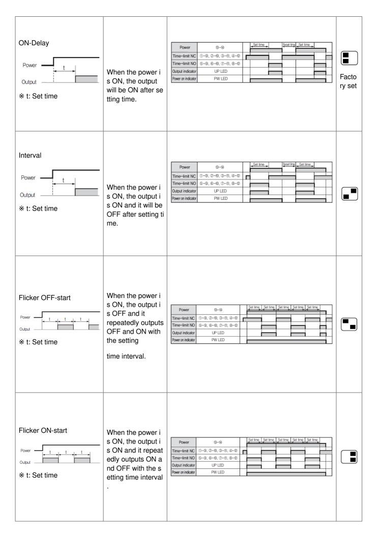
• Select output mode by 2 switches at the bottom of the four switches.
