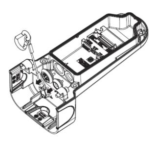
• Installing network cable (IP66)
