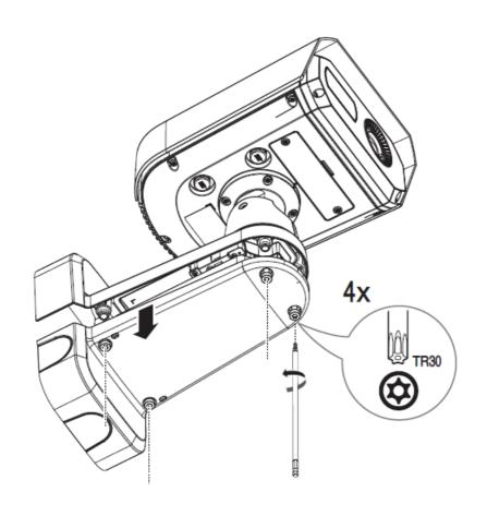
• When installing on a wall
