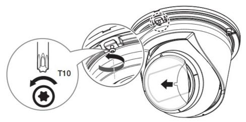
9. Push the colored camera part upward in the direction of the arrow, and tighten the screws in the direction perpendicular to the ceiling.
