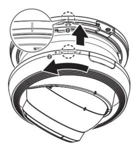
When connecting the cable through the side, remove the wiring hole cover first before doing so.
