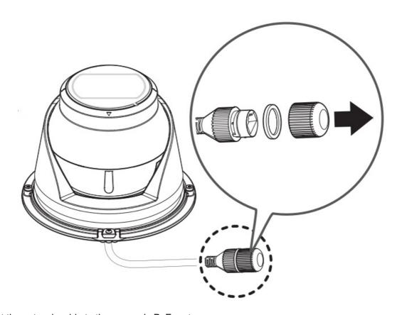
Connect the network cable to the camera's PoE port.
