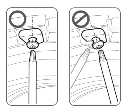
• Don't install the screws at an angle.
