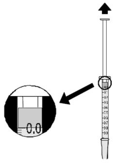
**Note:** To measure exactly 0.25 mL of the sample with the syringe, push the plunger completely into the syringe and insert the tip into the sample. Pull the plunger out until the lower edge of the seal is on the 0.0 mL mark of the syringe. Insert the syringe into the vial and push the reagent out until the lower edge of the seal is on the 0.25 mL mark.
