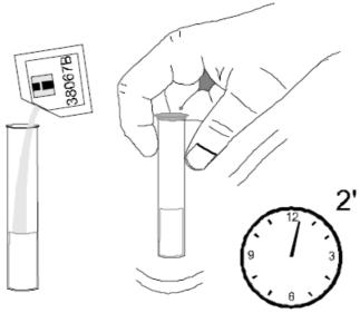
8. Remove the cap and add 1 packet of HI 38067C-0 reagent. Replace the cap and shake until the powder has completely dissolved.
