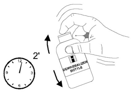
5. Flip open the top of the Demineralizer Bottle cap. By gently squeezing the bottle, add demineralized water to the other vial up to the 10 mL mark. Replace the cap and shake to mix.
