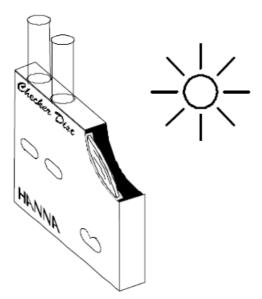
12. Keep the checker disc at a distance of 30-40 cm (12-16") to match the color. Rotate the disc while looking at the color test windows and stop when you find the color match.
