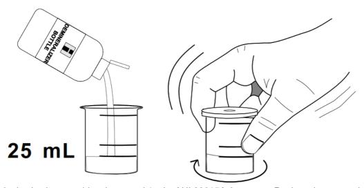
5. Using the 1 mL plastic pipette, add to the vessel 1 mL of HI 38015A-0 reagent. Replace the cap and swirl the vessel in tight circles to mix.
