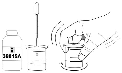
6. While swirling the vessel, add 10 drops of HI 38015B-0 reagent through the cap port. The solution will become a yellow color.
