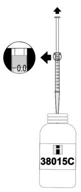
8. Place the syringe into the cap of the plastic vessel and slowly add the titration solution one drop at a time. Swirling to mix after each drop.
