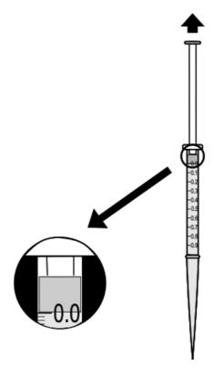
**Note**: To measure exactly 0.25 mL of sample with the syringe, push the plunger completely into the syringe and insert the tip into sample. Pull the plunger out until the lower edge of the seal is on 0.0 mL mark of the syringe. Insert the syringe into the vessel and push the sample out until the lower edge of the seal is on the 0.25 mL mark (the longer mark between 0.2 and 0.3).
