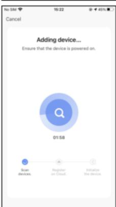
• AP mode: Click AP Mode, make sure your APP is internet available and device and APP both work in AP mode. Confirm to input the SSID and Password of Wi-Fi network, then select the Device AP name with SmartLife-xxxx in Wi-Fi list then back to App to finish the device adding.
