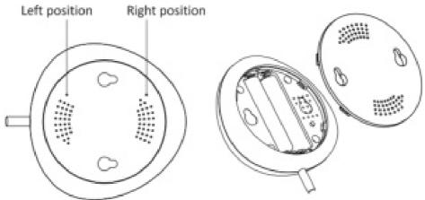
2. Put 2xAAA battery in with the correct positive and negative electrode.
