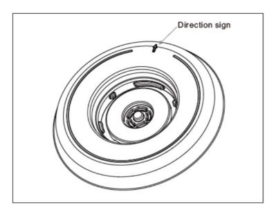
3. Place the plug part of the Sensor on the expansion interface and find the only installation position through 360° rotation. When rotating to the correct position, the module will be embedded downward. You can also refer to the direction guide arrow, and then rotate clockwise to complete the installation. When it cannot rotate any further, it is locked.
