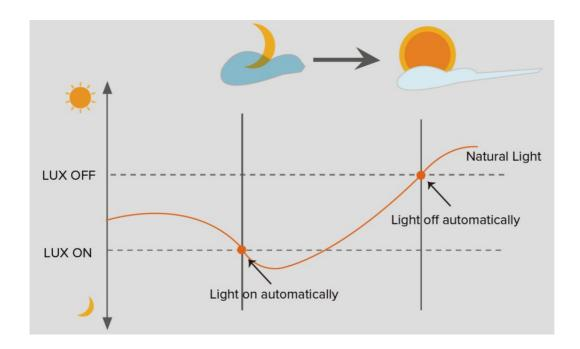
With Daylight Priority Function, HIGHBAY-MS is able to differentiate artificial light brightness from natural light after installed inside the fixture, and automatically turn off light when ambient brightness exceeds the preset Lux level.
