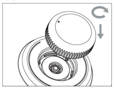
4. The installation should be carried out without power supply connected. Recheck and other relevant tests should be conducted after completion of the installation. After correct installation, the marking point of the Sensor shall be in the same direction as the interface direction arrow.
