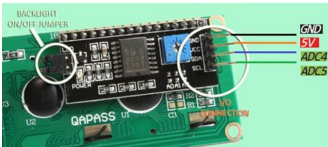
LCD display to Arduino wiring.
