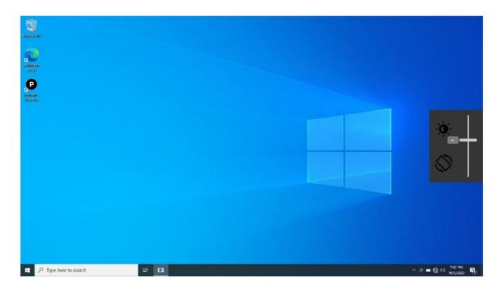
• Click the icon to switch between automatic dimming mode and manual dimming mode. In automatic dimming mode, the LCD will automatically adjust the brightness of the screen based on the background brightness. In manual dimming mode, use the right lever to adjust the brightness.
