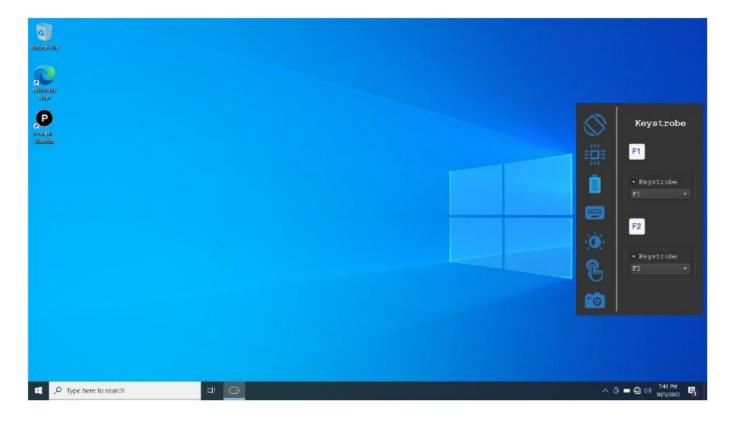
• The ALGIZ 10XR panel provides two user-defined function keys. Users can set the physical keys of the panel to any one of F1 to F12 according to their needs.
