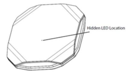
The AP351 Series access point is equipped with hidden LED display that indicates different status with different color. For the details of the LED status, please refer to the Quick Start Guide.
