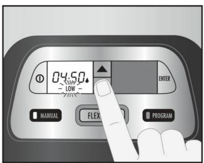
6. Press to turn off the slow cooker. NOTE: If is not pressed during the cycle, the unit will stay on the heat setting selected until the maximum cooking time of 24 hours is reached. Then it will turn off automatically.
