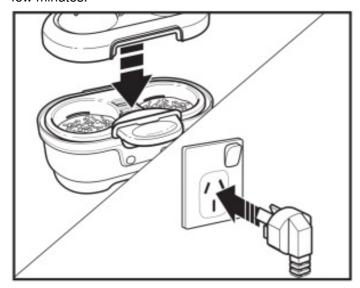
7. Unplug. Using oven mitts, lift Lid. Lift up Egg Tray by Handle and place on a heatproof surface.
