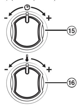
16. Temperature Dial ( → ) – Turn to adjust temperature from 170°F (77°C) to 450°F (232°C). Can be adjusted at any time.
