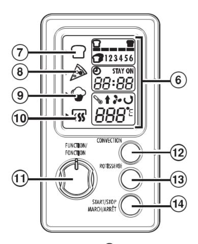
15. Time Dial with Auto Shut Off ( ) – Turn to adjust cook time from 1 minute to 4 hours, except in Broil mode. Timer has a stay on feature to use during~ and~ modes, CONVECTION and ROTISSERIE. STAY ON will be on the display. Can be adjusted at any time.
