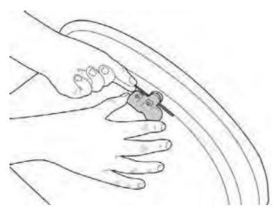
5. Hold the anti-rotation pin securely and use an 12 mm socket and torque tool to tighten the nut to 44.25 in-lbs.
