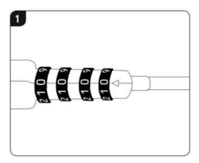
• With a valid combination (`0000' factory setting, or stored personal code), push the cable towards the numbered wheels and hold it in position. (Fig. 2)
