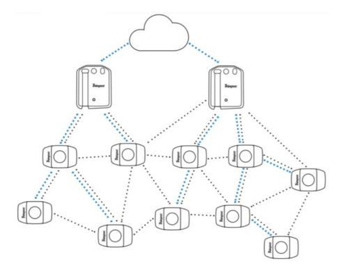
The amount sensors per one gateway varies depending on the sensors' reporting time: the longer the reporting time, the more sensor can be connected to one gateway. The usual amount is from 50-100 sensors per gateway to even up to 200 sensors.
