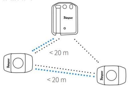
If the distance between a measuring sensor and the gateway is > 20m or if the sensors are separated by a fire door or other thick building materials, use extra sensors as routers.
