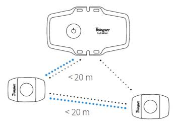
Install the gateway to a secure location. In public places, install the gateway behind locked doors. To ensure strong enough signal strength for data delivery, keep the maximum distance between mesh network devices under 20 m. If the distance between a measuring sensor and the gateway is > 20m or if the sensors are separated by a fire door or other thick building materials, use extra sensors as routers.
