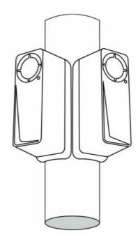
The main thing to consider when choosing the installation method is to ensure a clear view of the detection beam towards the observed area.
