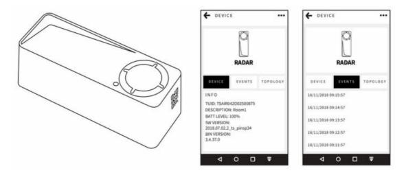
**Note:** Make sure the sensor is installed max. 20 meters from the next sensor or gateway. This is to ensure a full coverage mesh network between the sensors and the gateway.
