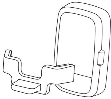
Hold the magnet switch tool against the sensor until the LED indicator starts to blink brightly for one minute. When the LED goes off, the sensor is switched on.
