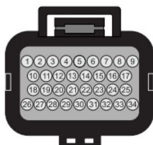
uC-10 Main connector AMP 34-pin Keyway 2 Wire side view
