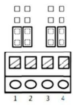
To configure input ports for contact closure, the jumpers should be placed vertically on the top two pins of each column of jumper pins, as shown below for the two ports. In this configuration, the state of the inputs will be closed ('1') until contact-closure occurs, at which point the input state will be open ('0').
