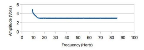
For AC signals at low frequencies the minimum input voltage becomes a function of frequency. The above graph depicts this relationship.
