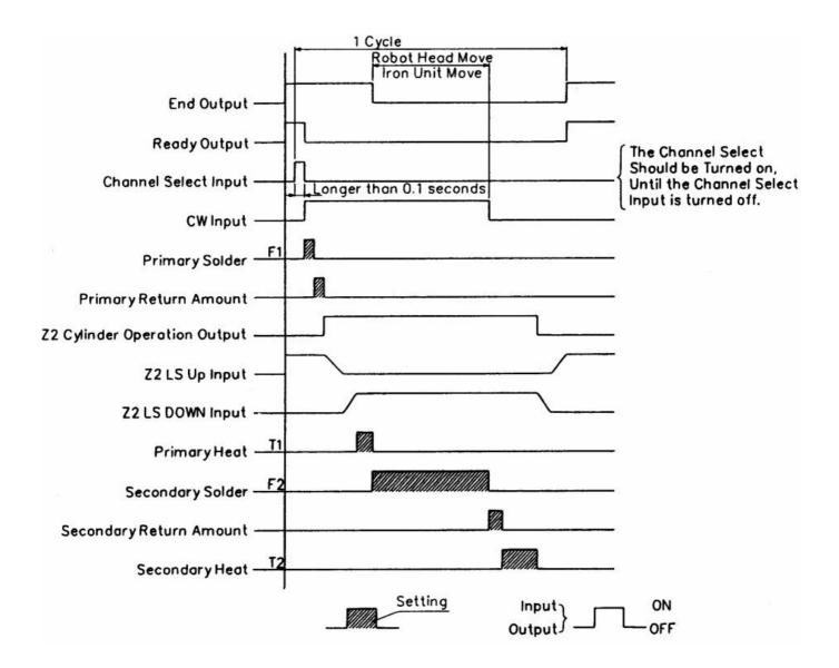
• During CW operation, the END and READY outputs are held OFF when there is an alarm.
