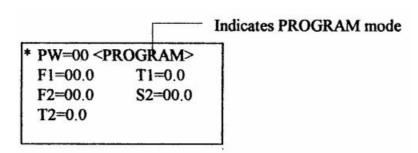
To change to PROGRAM mode, press the <MODE> key repeatedly until the word "PROGRAM" appears in the top right comer of the display.
