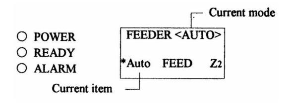
The current mode is displayed in the top right corner of the display. An asterisk (\*) is shown to the left of the current item. Use the <->> key to move the asterisk and select the desired item.
