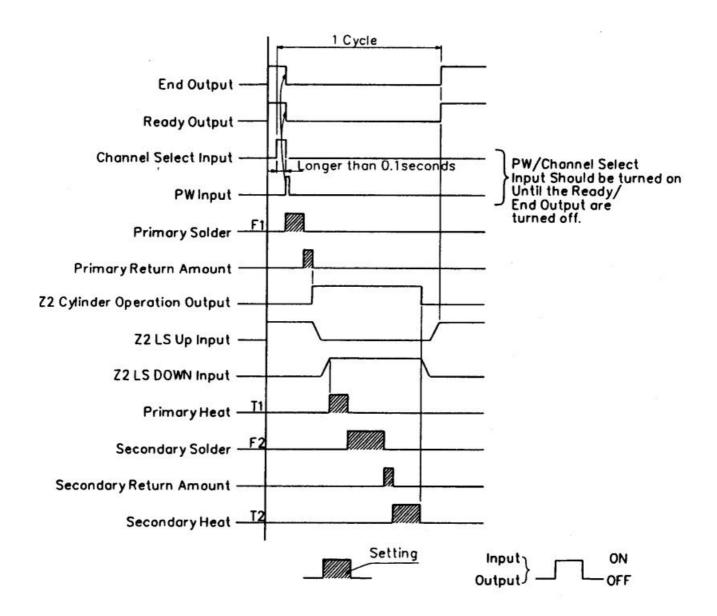
• During PW operation, the END and READY outputs are held OFF when there is an alarm.
