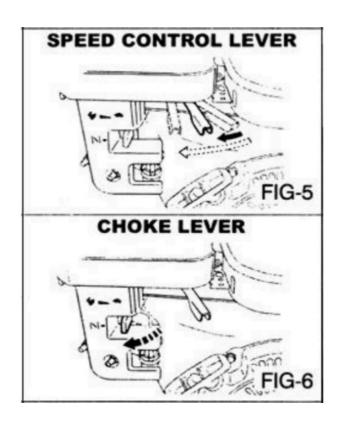
If the engine is cold or the ambient temperature is low, close the choke lever fully. (Fig-6) 3-5. Pull the starter handle slowly until resistance is felt. This is the "compression" point. Return the handle to its original position and pull swiftly. Do not pull out the rope all the way. After starter the engine, allow the starter handle to return to its original position while still holding the handle.(Fig-7)
