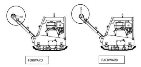
4-5. When shutting off the vibrator, turn the speed control lever from the HIGH to LOW position. Do not move the speed control lever slowly.
