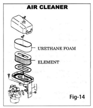
Dirty air cleaner element will cause starting difficulty, power loss, engine malfunctions, and shorten engine life extremely.
