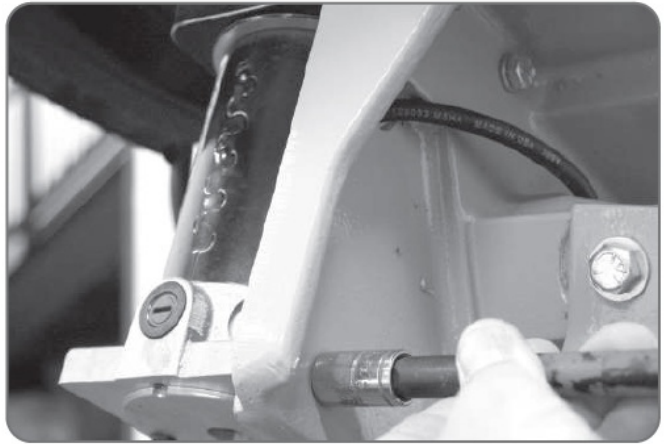
Figure 8 Shown using a 6" extension with 7/16" socket.
