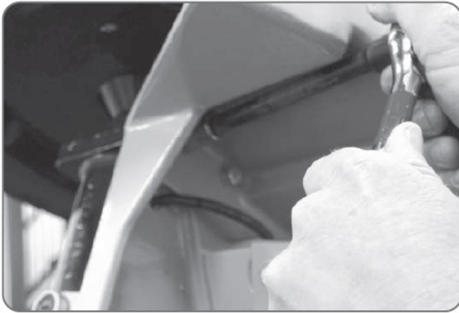
Figure 7 Shown using a 6" extension with 1/2" socket.
