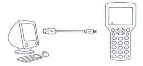
With a Micro USB cable to connect the device with the PC. When PC lower-left corner decoding mode, the device indicates a successful connection. Click 'start' to oper decoded.
