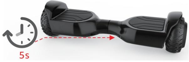
5. After a few seconds of resetting, the signal light and alarm will stop.
