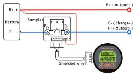
• Connection diagram of 100A/350A sampler
