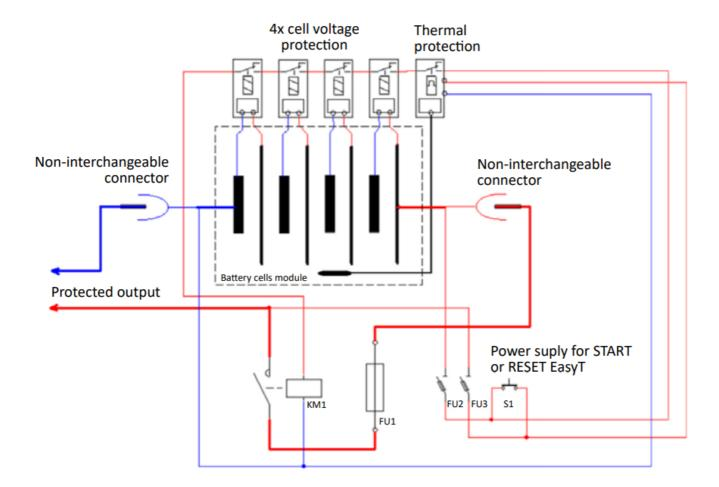
If a cell goes out of the allowed voltage range or the temperature of the cell block exceeds the allowed temperature, the relay on the corresponding Easy module switches to the NC position, and contactor KM1 loses voltage on the coil and disconnects the power.
