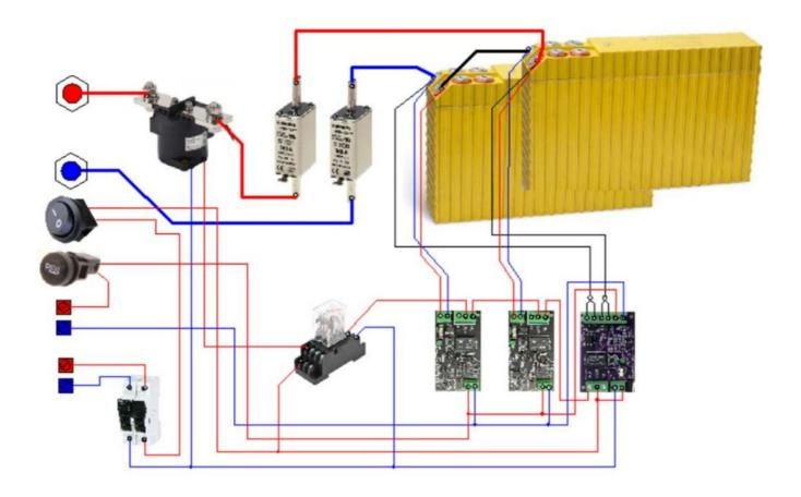
In more advanced systems, an independent 24V DC backup power supply for the control circuits is available. This can be used to power the EasyT module, the power contactor, and its auxiliary relay. The robust and durable BMS Easy system without software can have, for example, a basic (backup, emergency) function alongside of an advanced digital superstructure.
