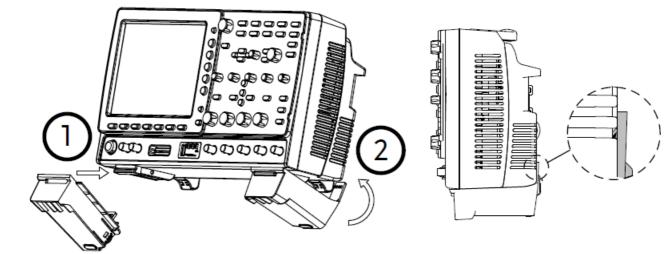
Installing the AFG-125/225 Module
