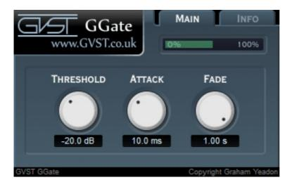
Three knobs control GGate's parameters. Each is clearly labelled above, with a user-editable readout below. Additionally, a meter provides visual feedback as to the activity level of the gate.
