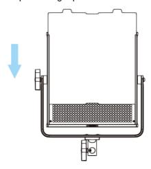
3. Loosen the adjustment knobs on both sides of the U-bracket, adjust the angle of the panel you need, and then tighten the adjustment knobs on both sides of the U-bracket.
