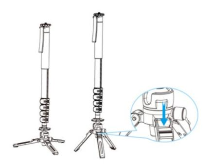
Press-tyoe button for gear adjustment
