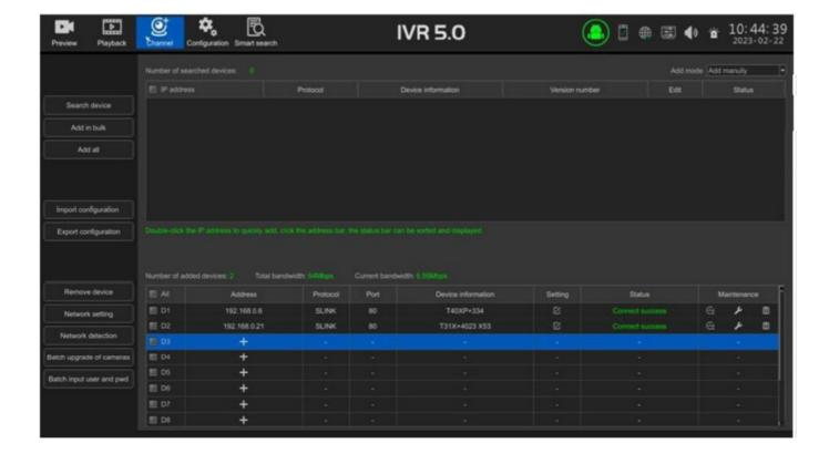
Click on "Search device" to automatically search for IP cameras within the local area network (LAN). The IP Monitor will detect and display a list of available IP cameras. You can choose to add them to the IP Monitor channels as required. Alternatively, if you have the specific IP address, port, and other camera parameters, you can manually input them and save the settings to add the camera to the IP Monitor.
