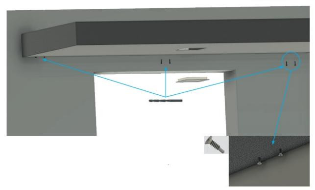
3. On the side where the side panel will be mounted, please use the countersunk screws (2x).
