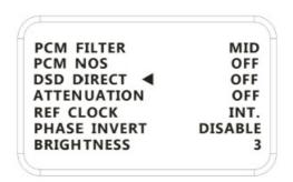
Default is OFF. Turn on to bypassing the internal interpolating FIR filter. The raw DSD stream is sent into the R-2R ladder directly.
