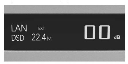
When selecting the external clock, if the external clock is lost, or the deviation of the external clock is greater than +- 1 5 0 p p m, it will display EXT ERR.
