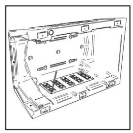
5. Using a 7/16" wrench or ratchet, emote the screws and washers fastening the upper and lower halves of the kennel.
