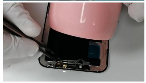
12. Remove the plastic protective film from the new screen
