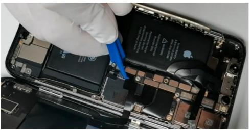
8. Connect the new screen cable to test the new screen for proper functionality before installation
