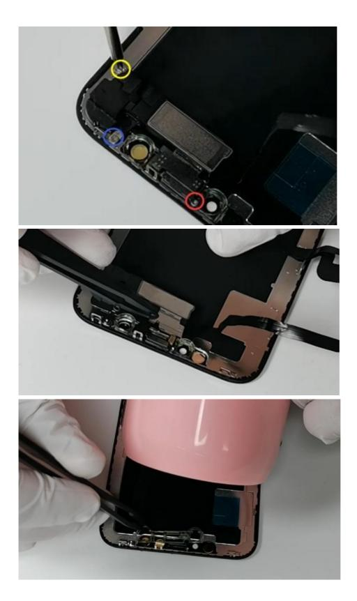
12. Remove the plastic protective film from the new screen  $% \left( 1\right) =\left( 1\right) \left( 1\right) \left$
