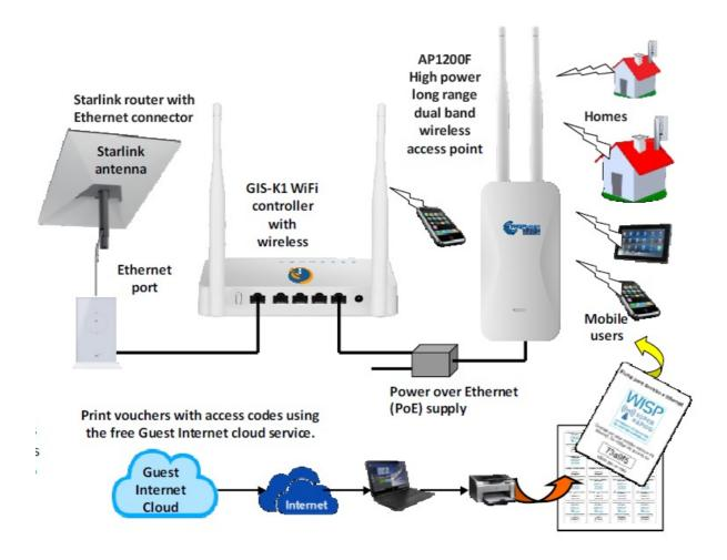
The AP1200F omnidirectional antenna is installed outdoors at a high point, such as the roof of a building. The installer has to provide the Ethernet cable that connects the AP1200F to the PoE supply.
