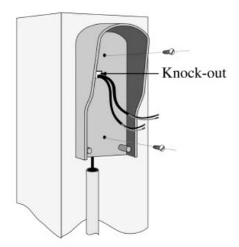
**Step 2:** To hard-wire the keypad – strip the wires back 3/16" and attach the wires to the terminal block marked RELAY OUTPUT on the keypad control board as shown to the right. Connect the other end to the opener's control board as shown in Control Board Connections section below.
