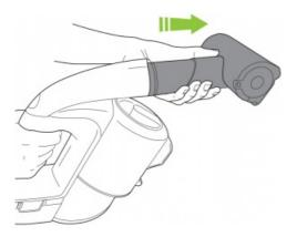
Gently pull the Power Brush from the Multi to remove. The battery should be removed when changing attachments.
