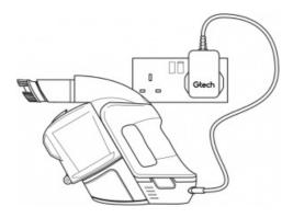
The battery can be charged on or off the main unit
