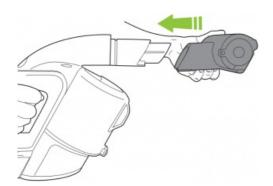
Make sure the terminals on the Power Brush and Active nozzle are correctly lined up and gently push the Power brush onto the Active nozzle. The battery should be removed when changing attachments.
