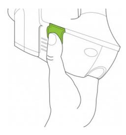
Press the green buttons and pull to remove the battery. The battery can be charged on or off the main unit. If you want to buy a spare battery go to <a href="https://www.gtech.co.uk">www.gtech.co.uk</a> or call **01905 345891**
