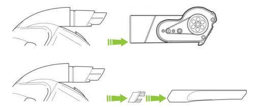
An active nozzle is built into your Multi. The dusting brush, crevice tool, and power brush all attach to the active nozzle.
