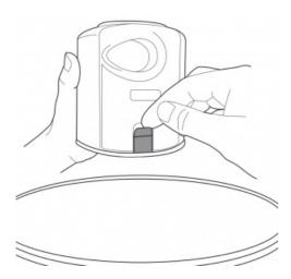
Hold the Multi's bin over a rubbish bin and release the latch to empty the dirt. A gentle tap will help. Remove the filter and tap off the excess debris each time you empty the bin.
