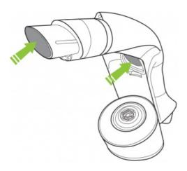
Remove the battery & bin and look through both ends of the tube. Remove any blockages.
