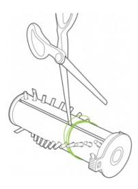
To remove hair from the brush bar, run an open pair of scissors down the groove to cut the hair, then pull it out. Never operate the power brush without the brush bar in.
