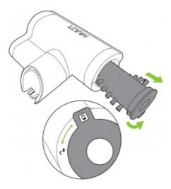
To clean the brush bar, first remove the power brush. Rotate the latch from the lock to the unlock position and pull out the brush bar.
