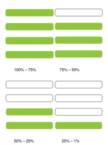
The battery state of charge indicator shows how much charge the Multi has. As you use the product, the green lights will turn off in a downwards direction.
