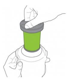
Remove the filter by pulling it from the top of the bin. Tap the dirt from the filter and tip any dirt from the filter housing. Wash the filter if necessary.
