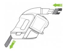
The dusting brush can be slotted onto the active nozzle. The crevice tool is stored on board the product for easy access.
