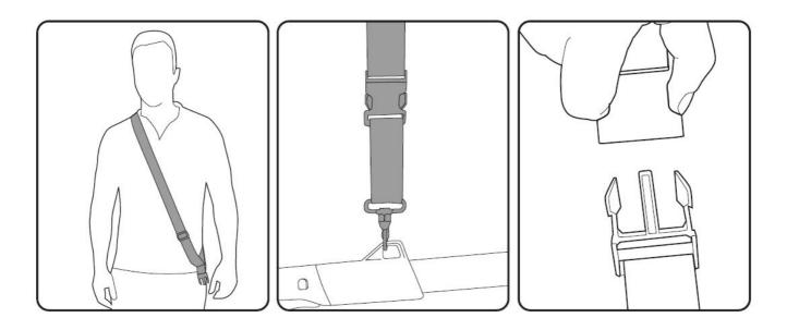
The harness is included as a safety feature for use with the branch cutter and the hedge trimmer. The sling passes over your head and rests on your shoulder – use the sliding adjuster to ensure the harness fits you comfortably. Attach the clip to the loop on the top of the handle. Then attach the clip to the harnesses. In an emergency situation, the harness clip can be released quickly.
