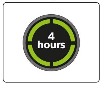
While charging, the LEDs will progressively pulse until all 4 are lit. The battery can be charged from flat in 4 hours. The state-of-charge indicator will show 4 solid green lights when it is fully charged.
