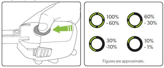
Press the button to check how much charge there is in the battery. The number of lit LEDs shows the charge.
