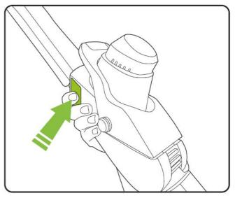
Remove the battery and ensure the cover is on the blade. Press the green buttons on either side of the trimmer head.
