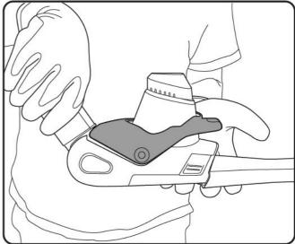
Remove the battery and ensure that the blade cover is on before continuing the next step. Depress the lever as shown. The head will now rotate freely. You can now rotate the head whilst pressing down on the lever. Release the lever and it will lock into place. This feature does NOT work with the branch-cutter.
