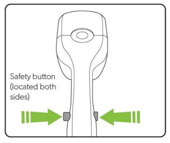
Push and hold the safety button on either side, then press the trigger to operate. When you release the trigger, the hedge trimmer will stop.
