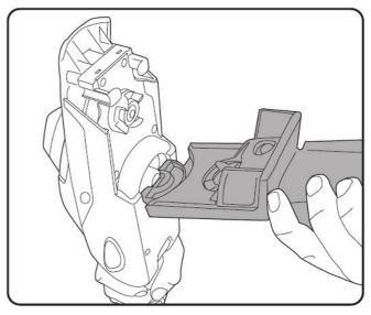
When the pole is fully inserted, the button (1) will pop up into the aperture (2). To remove, press the button (1) and pull the pole. With the blade cover still on, connect the hedge trimmer blade to the head.
