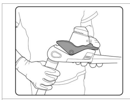
Remove the battery and ensure that the blade cover is on before continuing the next step. Depress the lever as shown. The head will now rotate freely.
