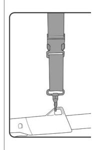
The harness is included as a safety feature for use with the branch cutter and the hed ge trimmer. The sling passes over your head and rests on your shoulder – use the slid ing adjuster to ensure the harness fits you comfortably.
