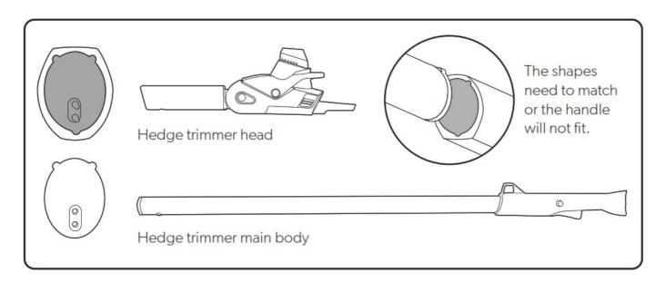
When inserting the body into the hedge trimmer head, ensure the body is the right way up. The shapes need to match or the handle will not fit.
