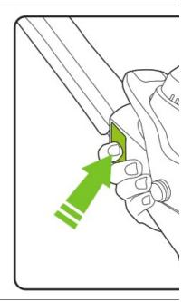
Remove the battery and ensure the cover is on the blade.
