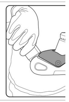
You can now rotate the head whilst press lever and it will lock into place. This featucutter.
