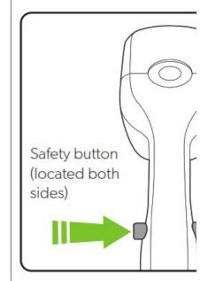
Push and hold the safety button on either side, then press the trigger to operate
