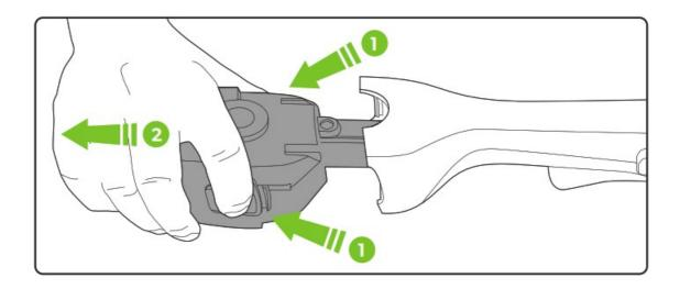
Press both buttons at the same time and pull to remove the battery.
