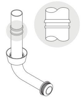
• Insert rubber clump, threaded stud and washers on supply pipe
