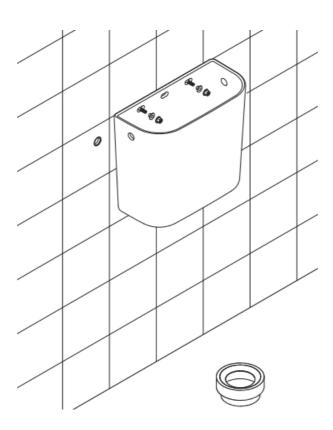
• Remove the diaphragm from the supply lateral hole and install the cistern
