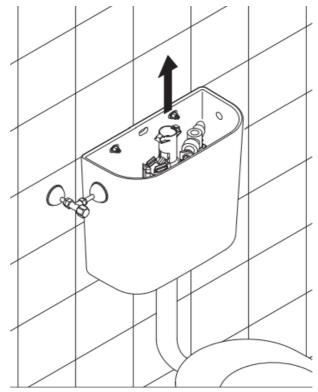
• Adjust the device height in order to suit the flush button and perform the hydraulic connections
