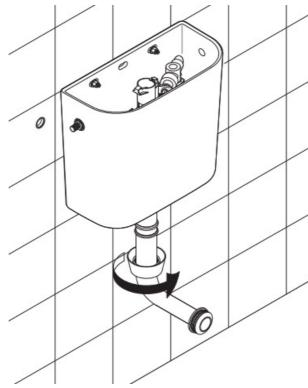
• Insert the pipe and screw the threaded stud
