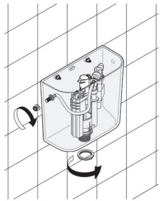
• Screw the flange and supply pipe
