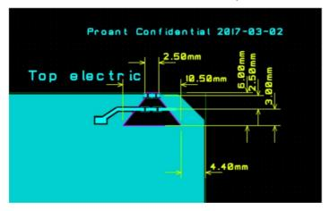
The antenna must be placed at the edge of the PCB, with appropriate grounding around the shape.
